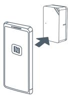
5. Basic information and settings of devices will be shown on ToolBox if it's recognized successfully. You can read and configure the device by tapping the Read/Write button on the App. In order to protect the security of devices, password validation is required when configuring via an unused phone. Default password is **123456**.
