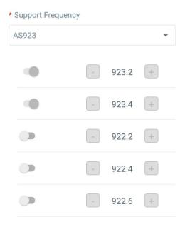
If frequency is one of CN470/AU915/US915, you can enter the index of the channel that you want to enable in the input box, making them separated by commas.
