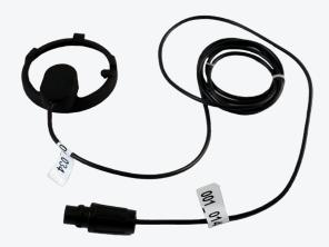
The inductive sensor is designed to transmit data from analog water meters to the Jooby OMNI RM LoRaWAN 4PU 200 / 204 / 205 EU Pulse Radio Module. The device is installed on the enclosure of the metering device and connected to the radio module. After that, the Sensor begins to record the number of revolutions of the water meter's measuring arrow and then transmits the data to the Pulse Radio Module.
