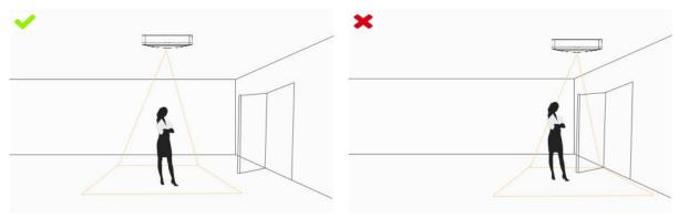
Avoid installing the sensor near a mirror or avoid drawing the line to the mirror.
