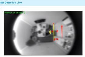
2) Ensure that the detected targets can pass through the detection line completely. It's recommended that the detection line is perpendicular to the In/Out direction and on the center of detection area without other objects around.
