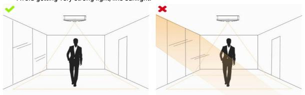
• Make sure there are no moving objects interfering in the counting area. For example, do not install the sensor too close to a door.
