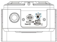
**Step 2:** Use mobile devices or laptop to connect to the device's Wi-Fi. **Note:** The Wi-Fi name is **SC311\_xxxxxx** (xxxxxx is the last six bits of the MAC address).
