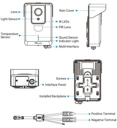
**Note:** The Positive Terminal of the solar panel cable needs to be connected to the Negative Terminal of the solar panel, and the Negative Terminal needs to be connected to the Positive Terminal of the solar panel.
