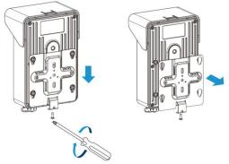
**Step 2:** Fix the backplane in the position where the device is intended to be installed. Multiple installation methods are available depending on the installation location:
