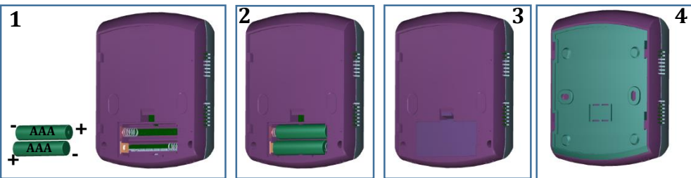
Picture 8. Steps to insert the batteries and then to assemble the device
