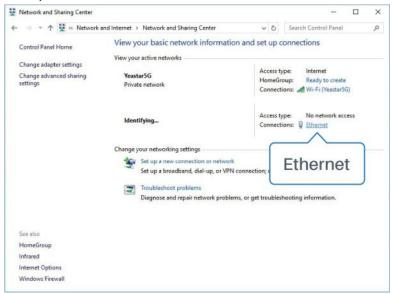
B. Go to "Properties" → "Internet Protocol Version 4(TCP/IPv4) ", select "Obtain an IP address automatically" or "Use the following IP address", then assign a static IP manually within the same subnet of the device.
