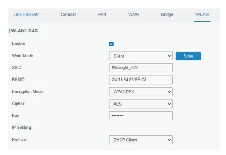
D. Go to "Network" → "Interface" → "Link Failover" to enable WLAN.
