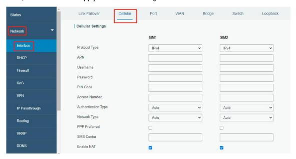
B. Go to "Network" → "Interface" → "Link Failover" to enable SIM1 and rise link priority of SIM1.
